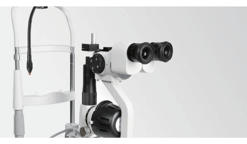
Classic Galilean type microscope Total magnification ratio: 6X,10X,16X,25X,40X Max.aperture diameter: Ø14mm Convergence angle of eyepieces:13° Excellent stability,available with applanation tonometer,digital camera,CCD,teaching tube,etc.
